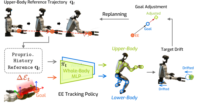
Fig. 2: HERO is an accurate end-effector control framework. Given an EE goal pose, HERO first uses IK to convert it into an upper-body goal. It then uses motion planning to generate an upper-body reference trajectory that is tracked via a learned tracking policy \pi_t (Sec. III). In addition to reference joints, \pi_t also takes accurate estimates of the residual EE error (obtained via a learned neural forward model (Sec. III-B, Sec. III-B2)). HERO also employs periodic replanning (Sec. III-C) to adapt to drifts and goal adjustment (Sec. III-D) to mitigate systematic tracking errors. Accurate tracking enables building modular object manipulation systems (Sec. IV, Fig. 3).
